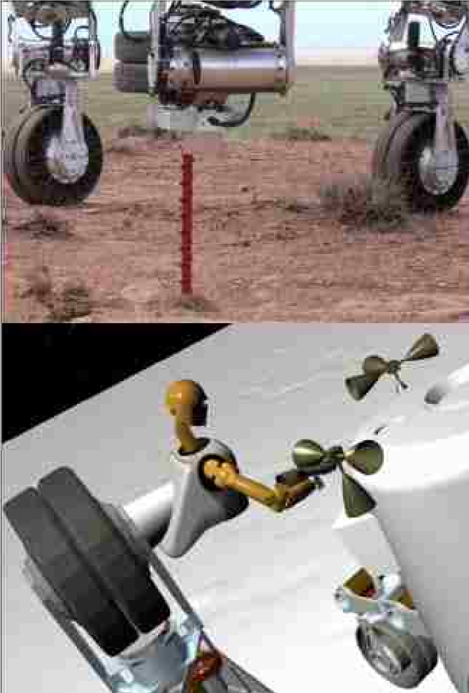
Top - ATHLETE drilling tool in natural terrain
