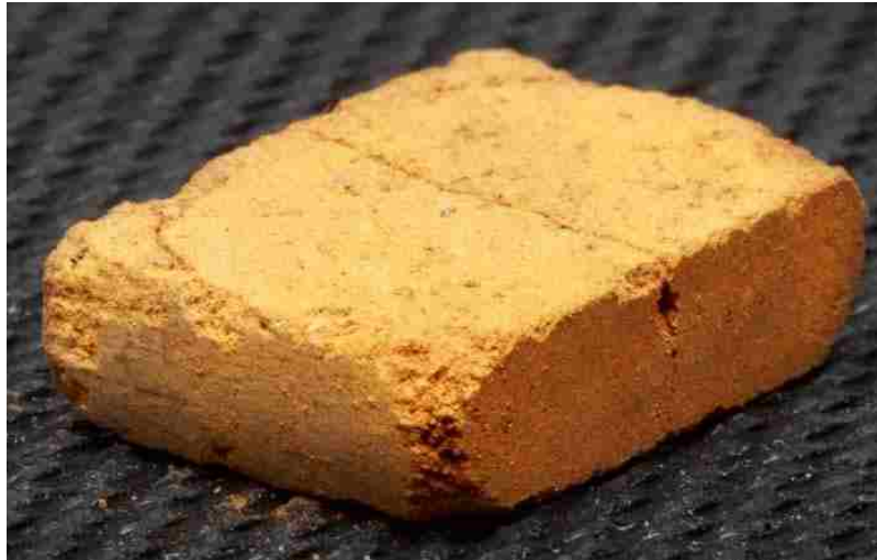
Figure 14: Processed Simulated Martian Soil Brick (Grush, 2017 [David Baillot])
